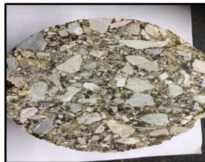
Section of BSM1-AGG compacted layer core (Bridgemohan, 2018)
